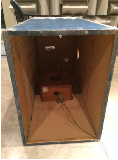
Figure 3.3 Photograph of loudspeaker inside of partial enclosure.
